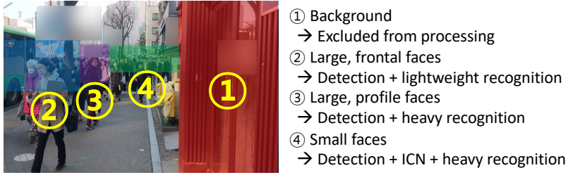
Figure 4.7: Operation of EagleEye in a nutshell.
