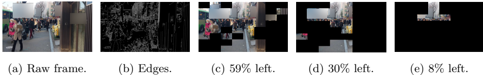
Figure 4.22: Example operation of Edge-Based Background Filtering.
