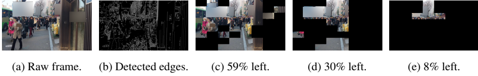
Figure 4.22: Example operation of Edge-Based Background Filtering.
